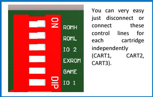
You can very easy just disconnect or connect these control lines for each cartridge independently (CART1, CART2, CART3).
